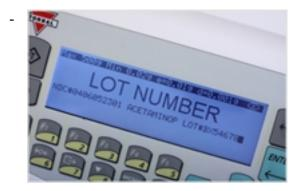
The pharmacist can assign a LOT number to a drug with the external PS/2 keyboard, which is very helpful in maintaining the average piece weight.
