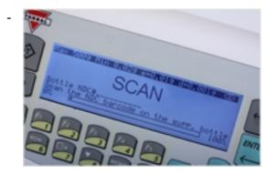
A large pixel LCD display shows full - text onscreen instructions and graphics while counting. A short wizard leads the leads the user through the simple pill counting operation.
