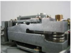
The heart of a quality is its load cell and suspension. The load cell should be of the electromagnetic force restoration type where the weight of the unknown is balanced out by the force generated by sending an electric current through a coil which is sitting in a high level magnetic field. The suspension should be of the Roberval type which compensates for end and side loads and allows the scale to be top loading.
